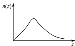
Fig. 10.10 Electron density in triangular potential well.
